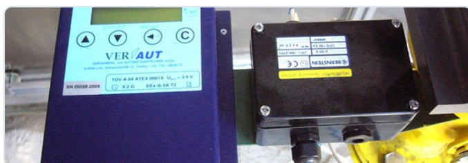
VERIBOX-MINI on a gas line, enclosure sealed
